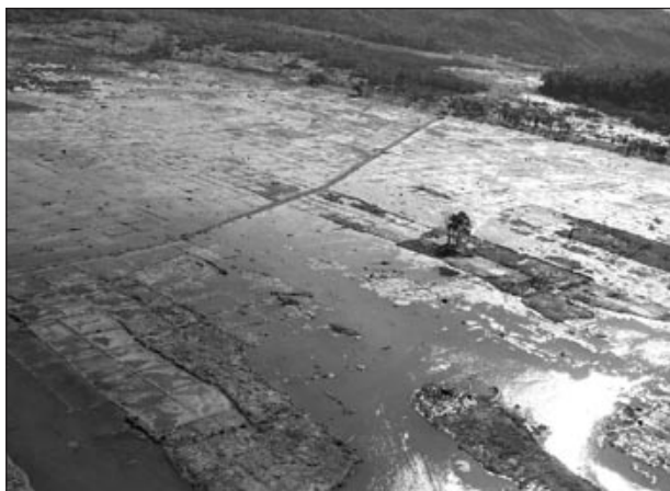
FIGURE 1 Aerial view of western Aceh Province near Calang showing the effects of tectonic subsidence.
