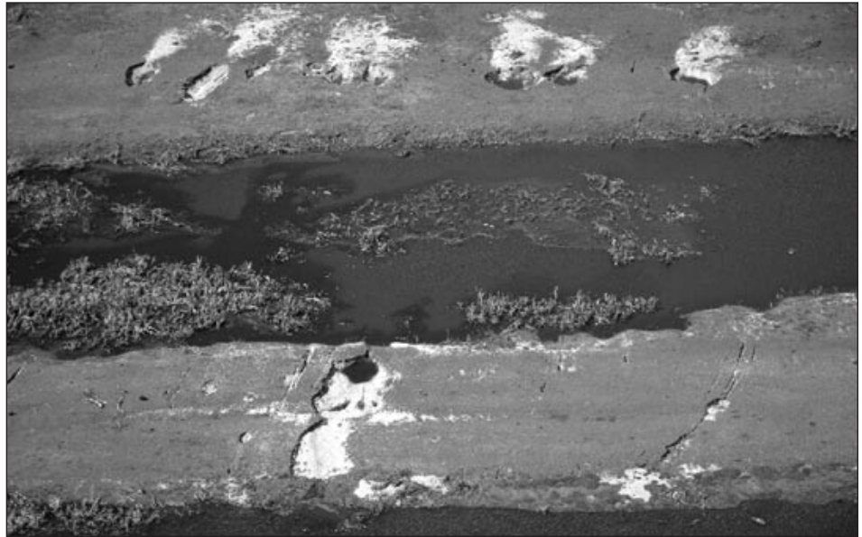
FIGURE 7 Aerial view of a coastal region north of Meulaboh showing coastal plain underlain by water-saturated loose deposits of beach sand that had experienced liquefaction. Sand blows were scoured by tsunami wave action.
